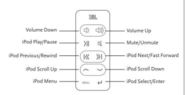
IBL 10-Button Remote Technical Specifications Transmission: 38kHz Frequency: Operating Range: 20 feet Battery Type: CR2025 3V Dimensions: Width: 1.29"(33mm) Height: 3.38" (86mm) 0.23" (6mm) Weight (including battery): 1.2 OZ.
